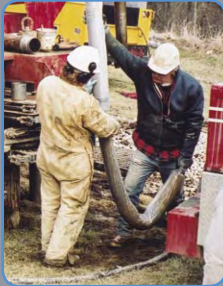
■ Extruding core sample using vibratory action.
