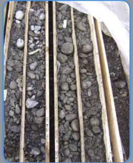
■ Core samples of gravel aquifer in core boxes ready for storage.
